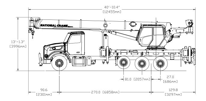
The configurations are based on the NBT45-2 with an 85% stability factor. The complete unit must be installed in accordance with factory requirements and a test performed to determine actual stability and counterweight requirements since individual truck chassis vary.
