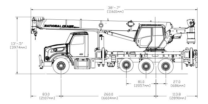
The configurations are based on the NBT40-2 with an 85% stability factor. The complete unit must be installed in accordance with factory requirements and a test performed to determine actual stability and counterweight requirements since individual truck chassis vary.
